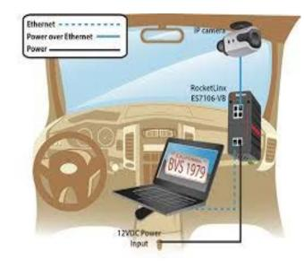
LPR is a completely hands-free approach to patrolling parking areas, as the cameras validate while driving. Data is immediately captured, cross referenced, and the officer is alerted if a violation is located.
